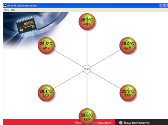
Fig.5: Snapshot of simulation scenario representing temperature and battery voltages of all the EDs along with AP
