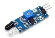
An electronic device that emits in order to detect some aspects of the environment is known as an infrared sensor. In addition to detecting motion, an IR sensor can also measure an object's heat. A passive IR sensor, on the other hand, measures only infrared radiation rather than emitting it. In most cases, all objects emit some kind of thermal radiation in the infrared spectrum. An infrared sensor can pick up these kinds of radiations, which aren't visible to our eyes but can
