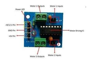
L293D is a common Engine driver or Engine Driver IC which permits DC engine to drive on one or the other course. The 16-pin IC known as L293D is capable of simultaneously controlling two DC motors in any direction. This indicates that a single L293D IC can be used to control two DC motors. Integrated circuit (IC) with two H-bridge motor drivers.
