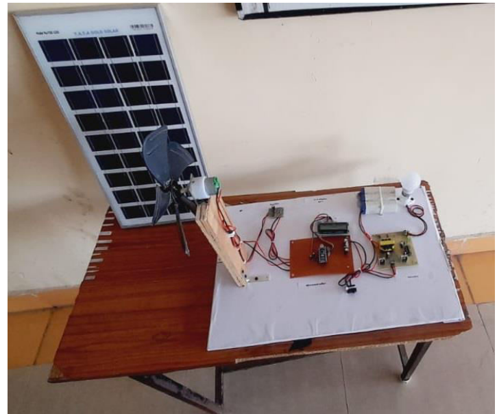
IV (a) Model of Hybrid Power Generation using Solar And Wind Energy to produce uninterrupted Electric Power
