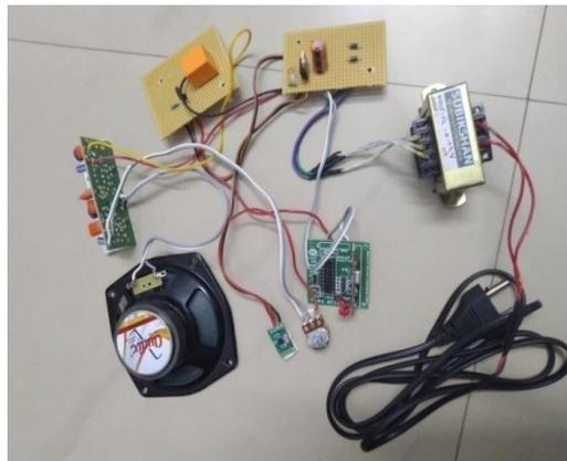
Fig 6. Switching Controller with Speaker Setup
