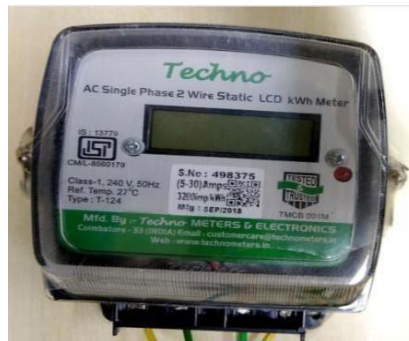
Fig.3 Digital energy meter
