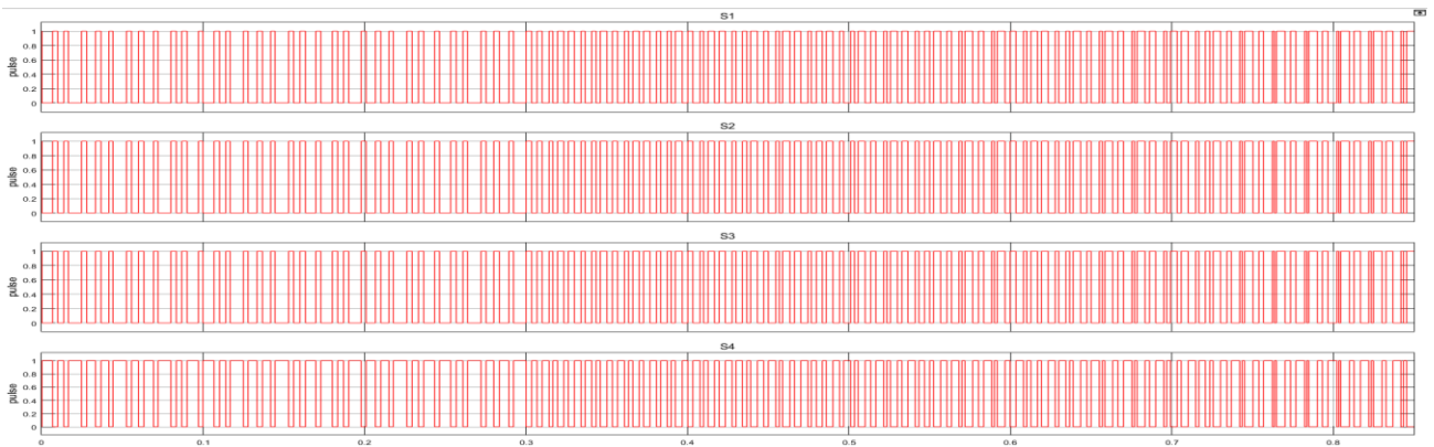
Fig.4. Switching signal obtained by minimum voltage algorithm
