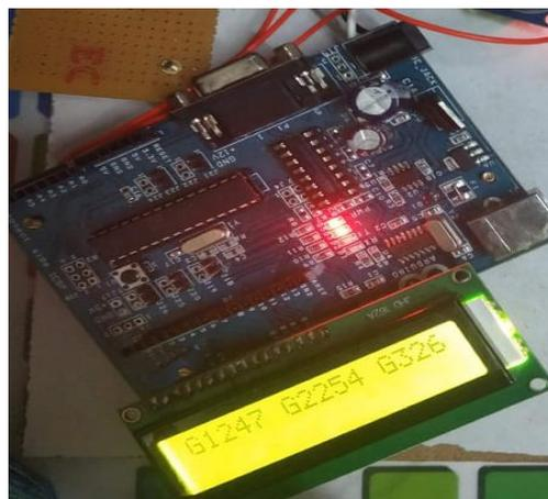
Fig 3(b) LCD Shows the Gas concentration
