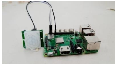
Fig1 PIR sensor and raspberry pi-3 Interface
