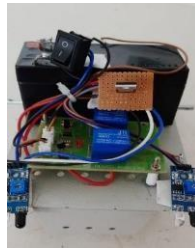
Fig3 Relay Board with IR Sensor and motor
