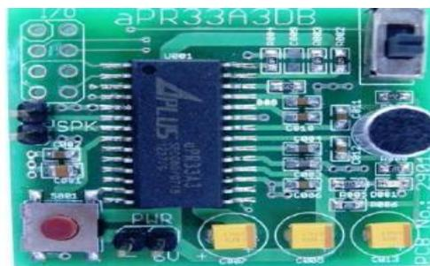
Figure 4. Voice recording/Playback unit
