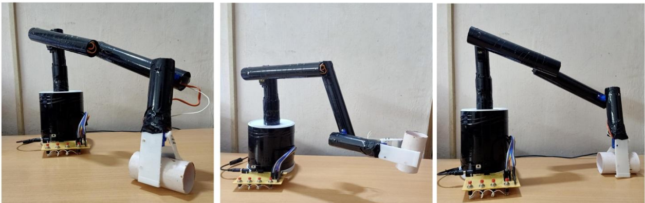
Fig.6: Execution of Pick and Place operation (Action Mode)
