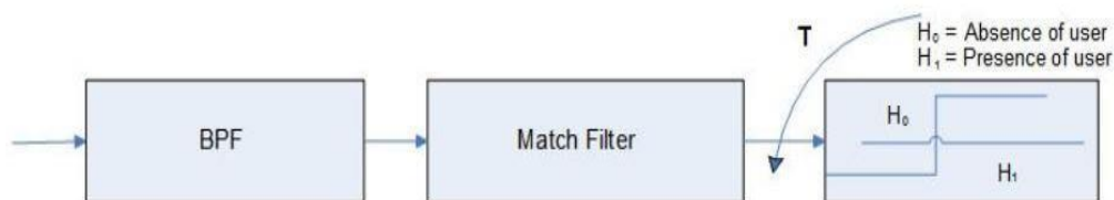
Figure 4: block diagram of matched filter detection
