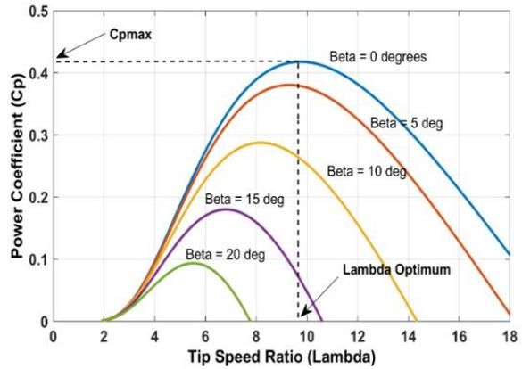
Fig.9.  $C_p$ - $\lambda$  characteristics for different pitch angles
