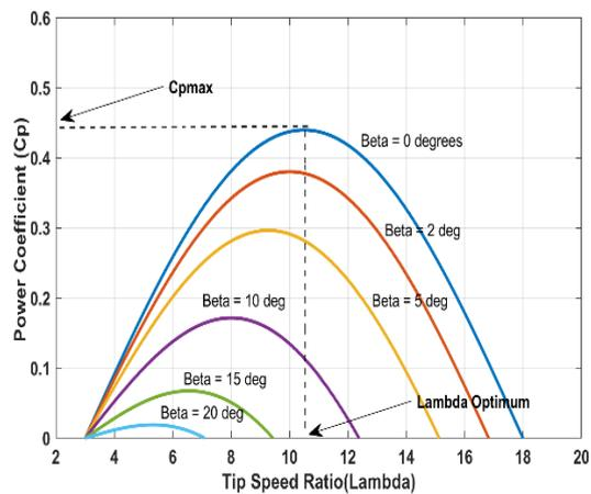
Fig.12.  $C_p$ - $\lambda$  characteristics for different pitch angles
