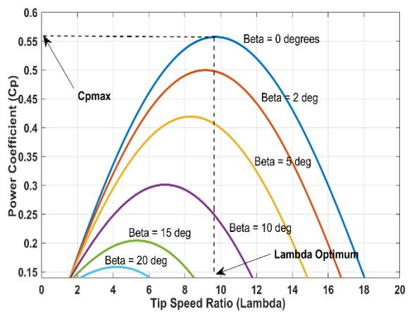
Fig.13.  $C_p$ - $\lambda$  characteristics for different pitch angles
