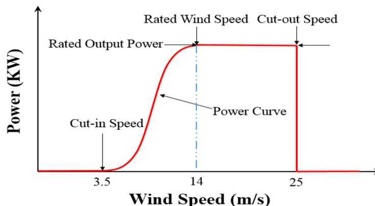
Fig.14. Typical wind turbine power curve showing three speeds
