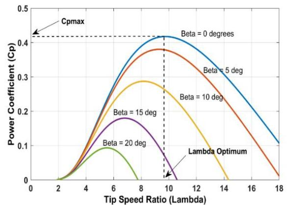
Fig.11.  $C_p$ - $\lambda$  characteristics for different pitch angles
