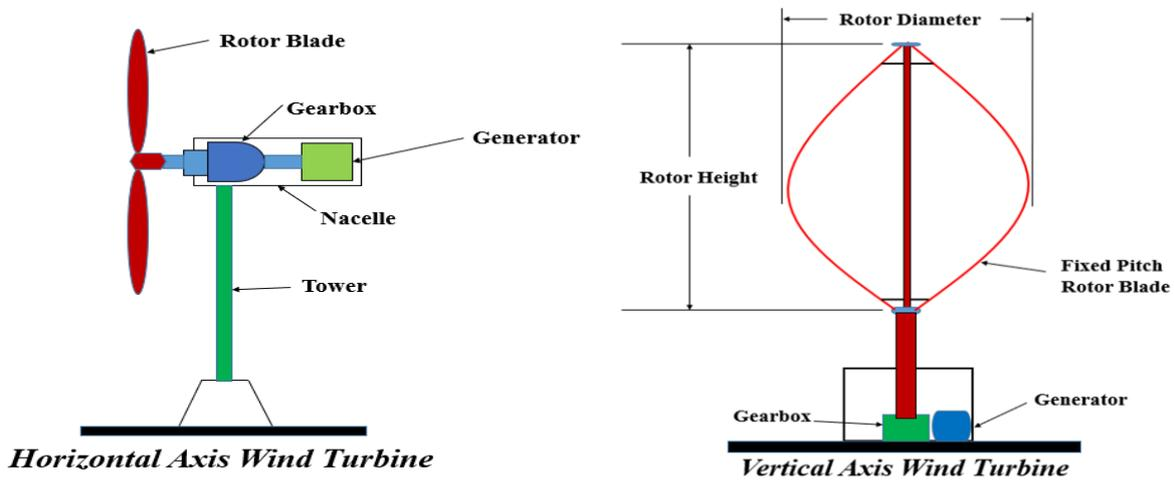
Fig.3. Types of wind turbines based on axes
