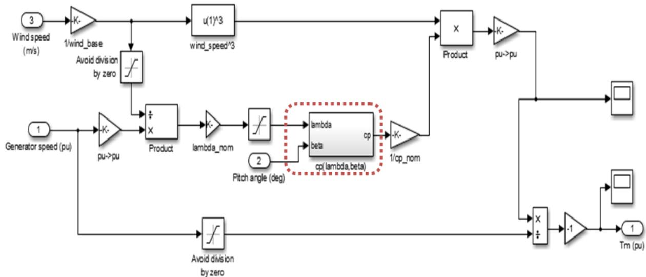
Fig.15 Simulation model for a wind turbine
