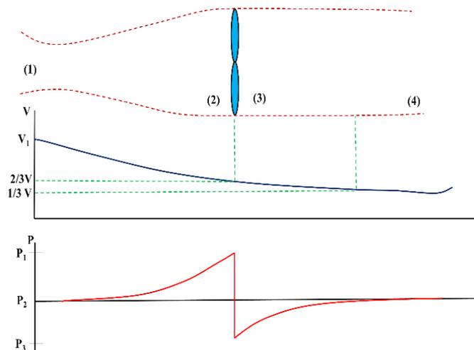
Fig.6. Packet of air moving with speed( $v$ )
