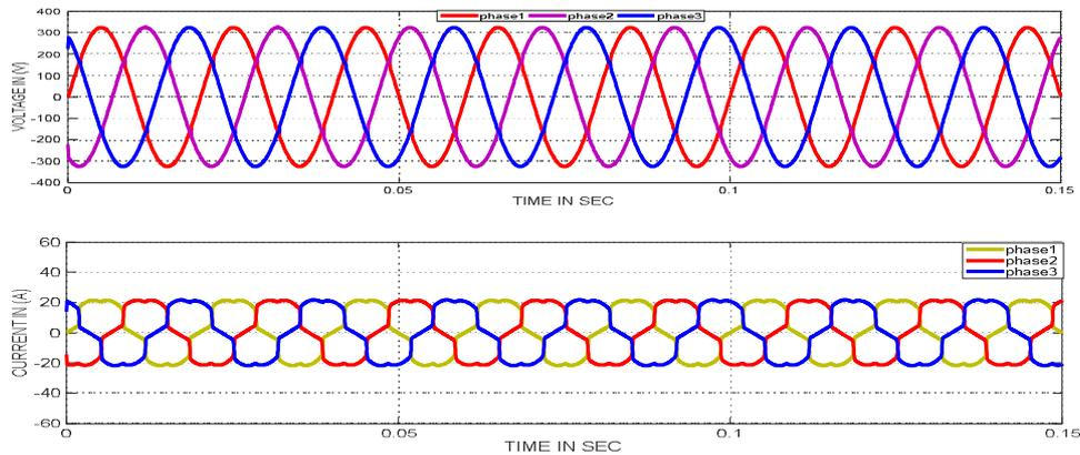
Fig. 9 Voltage and Current Waveform with C-types high pass filter Harmonic Filters.
