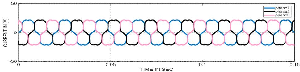
Fig. 11 Voltage and Current Waveform with C-types high pass + Double tuned passive Harmonic Filters.
