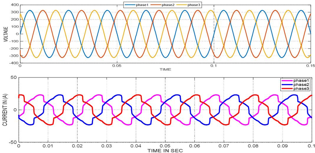
Fig. 3 Voltage and Current Waveform without Filters.
