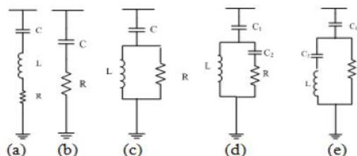
Fig. 1. Single-tuned (b) 1st order high-pass (c) 2nd order high-pass (d) 3rd order high-pass (e) C-type. [3]
