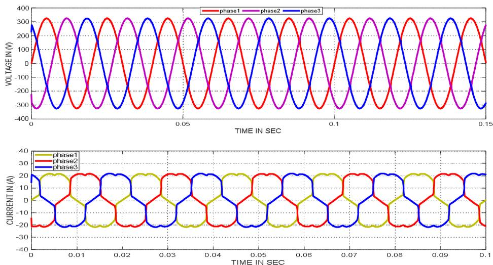
Fig. 5 Voltage and Current Waveform with Double Tuned Harmonic Filters.
