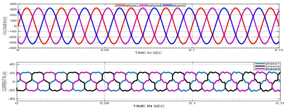
Fig. 7 Voltage and Current Waveform with Single Tuned Harmonic Filters.
