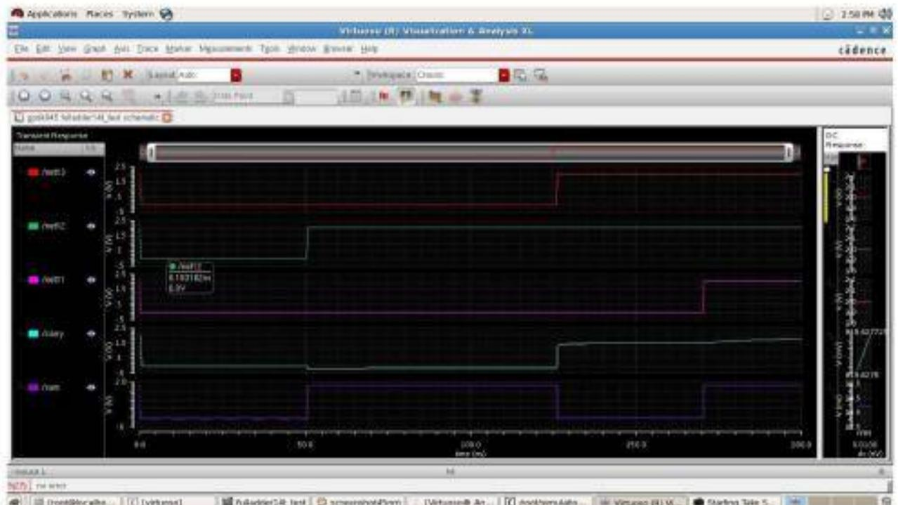
Fig.4.4.: Transient response of 14t full adder
