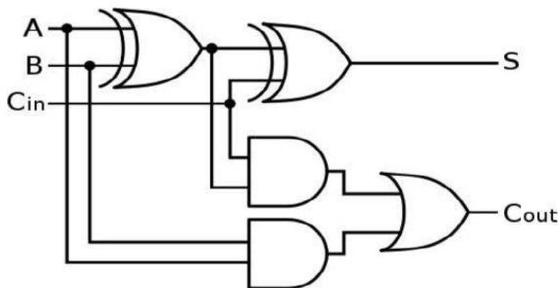
Fig.3.1.: Logic diagram of full adder
