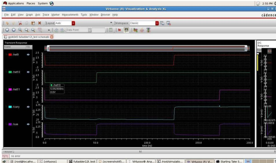
Fig.4.3.: Transient response of 12T full adder
