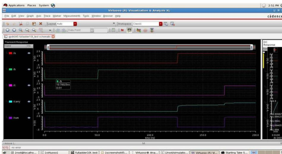
Fig.4.2.: Transient response of 10T full adder
