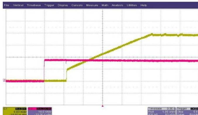
Fig. 9 12V System, 20A Load. Red: Input voltage, Yellow: Output current
