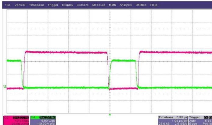
Fig. 7 12V system, 20A load. Top and bottom gate waveforms show dead-time implementation.
