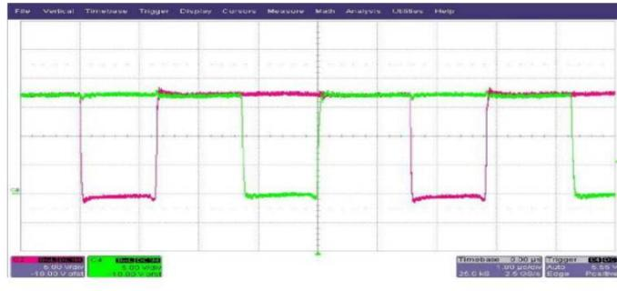
Fig. 8 12V system, 20A load Individual channel switch nodes show interleaved operation
