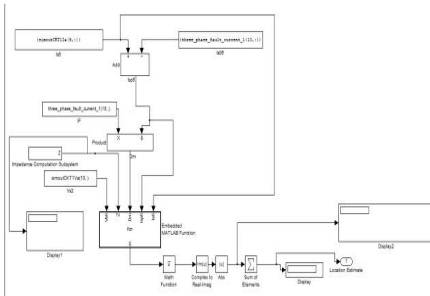
Figure 3: Fault location subsystem.
