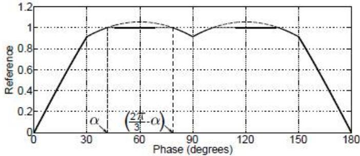
Fig. 6. Clipped reference signal and angle  $\alpha$  in over-modulation region 1
