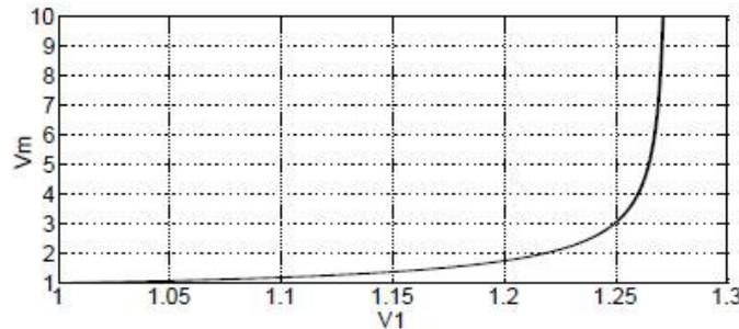
Fig. 3. Peak reference fundamental versus peak output fundamental
