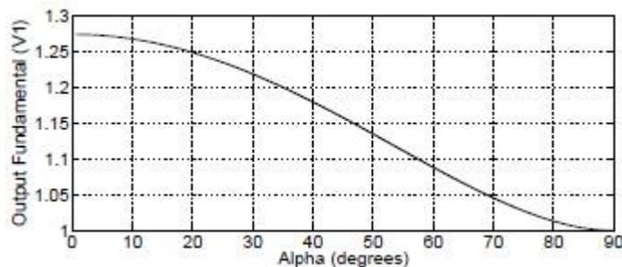
Fig. 2. Output fundamental versus  $\alpha$  - SPWM
