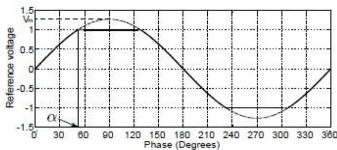
Fig. 1: Limiting of reference voltage in over-modulation region
