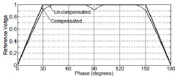
Fig. 7. Reference Voltage for MI=1.218
