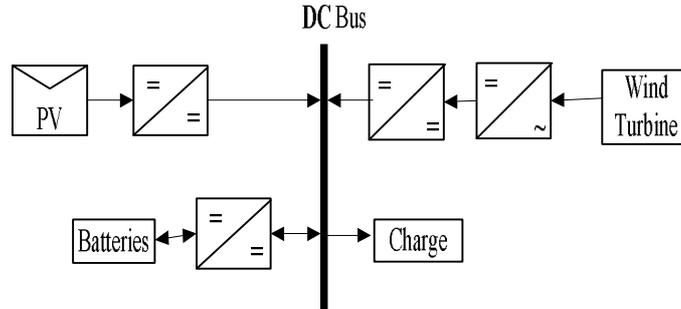
Fig. 1. Schematic of the Hybrid-RES system
