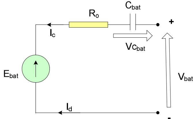
Fig. 3. Equivalent circuit diagram of a cell of the Nickel-Cadmium Battery
