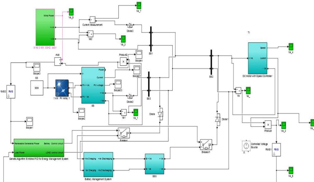
Fig. 7. Developed Hybrid-RES system comprising Wind-Turbine and Photovoltaic Cells
