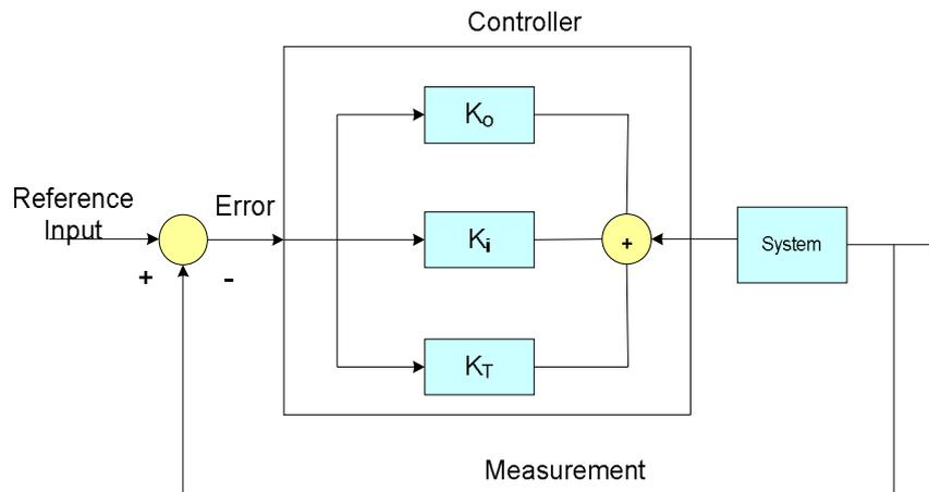
Fig. 4. Schematic of PID controller
