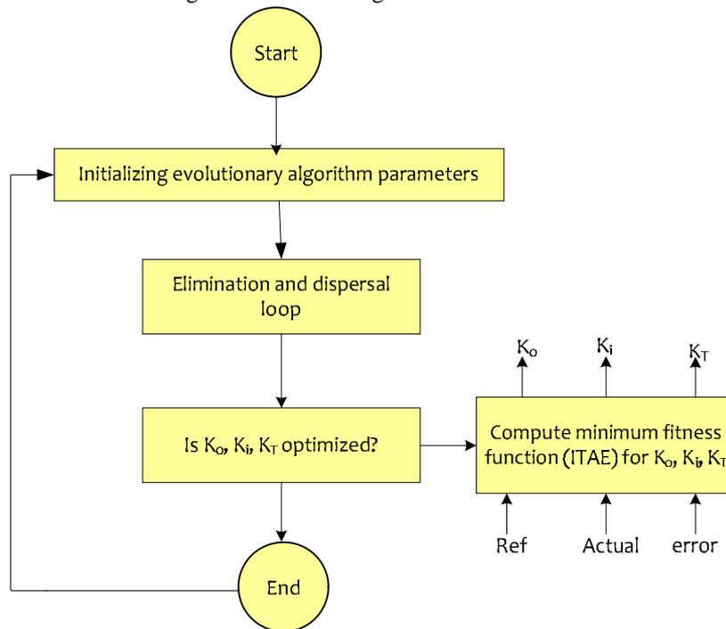
Fig. 5. Evolutionary Computing based PID parameter tuning for load sensitive EMS control
