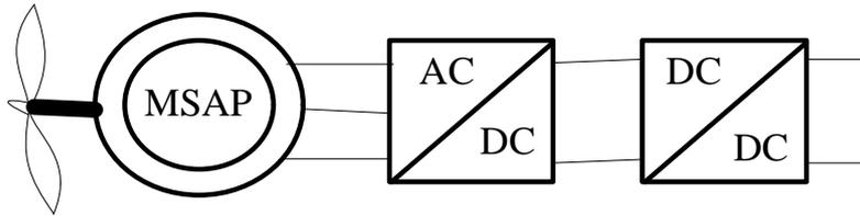
Fig. 2. Wind Turbine Energy Conversion System
