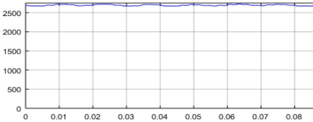
Fig. 14. WECS generated power (W) with BPSO-PID controller
