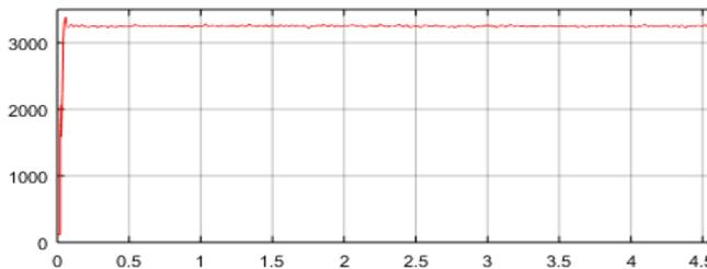
Fig. 10. Hybrid-RES generated power (W) with classical PID control
