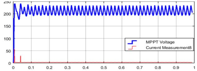
Fig. 15. Voltage (V) and Current (A) generated from PV cell using BPSO-PID assisted RES system
