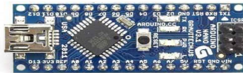
Figure 1. Hardware Architecture of Arduino NANO
