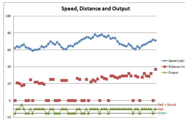
Figure 5. Point-to-Point Relation of Speed, Distance and Output of (a) City Road Testing and (b) Highway road testing
