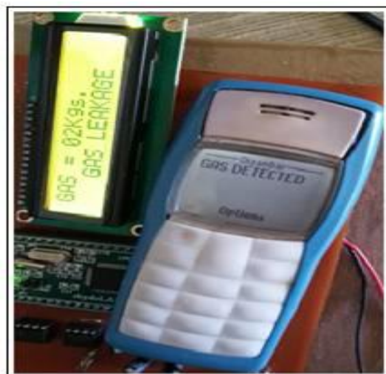
Fig.4: Gas Leakage Detected
