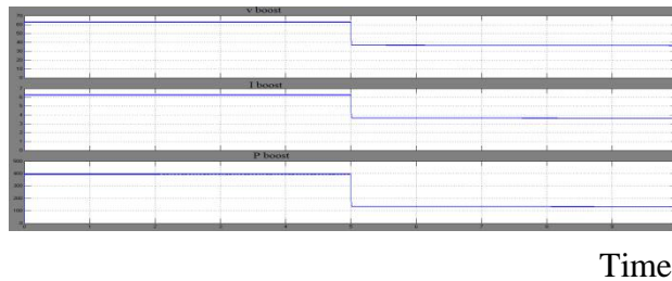
Fig. 8 Output voltage waveform of boost converter at irradiation level of 1000W/ and 500W/
