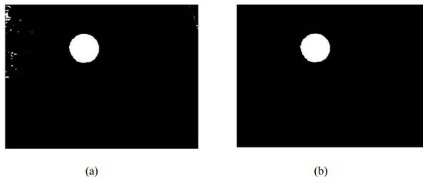
Fig. 4: (a) Before removing small areas (b) After removing small areas
