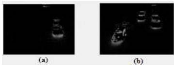
Fig.3 Moving Object Detection with Output of FD with binary thresholding (a) one car (b) more than 1 car.
