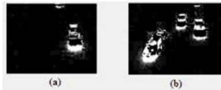
Fig.4 Moving Object Detection with Output of FD with adaptive thresholding (a) one car (b) more than 1 car.
