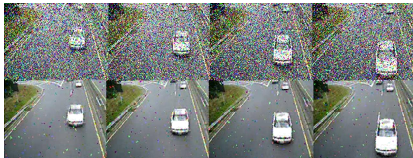
Fig. 3: Results obtained for the noise corrupted video frames with 30% noise density and its corresponding denoised frames (top four frames are noise frames and corresponding bottom frames are denoised frames).
