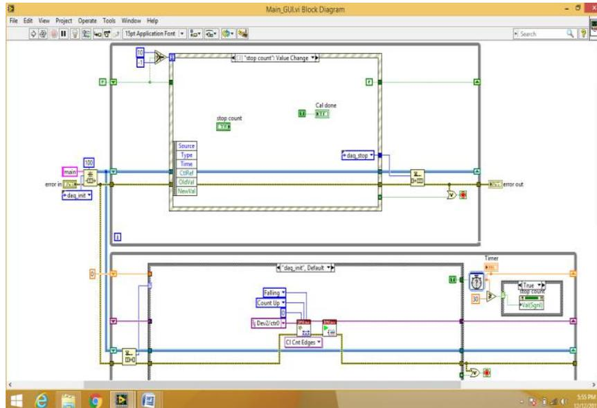
Fig 2. Design of Pulse Wave Record in LabVIEW
