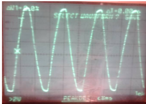
Fig 9 Output Waveform without compensator
