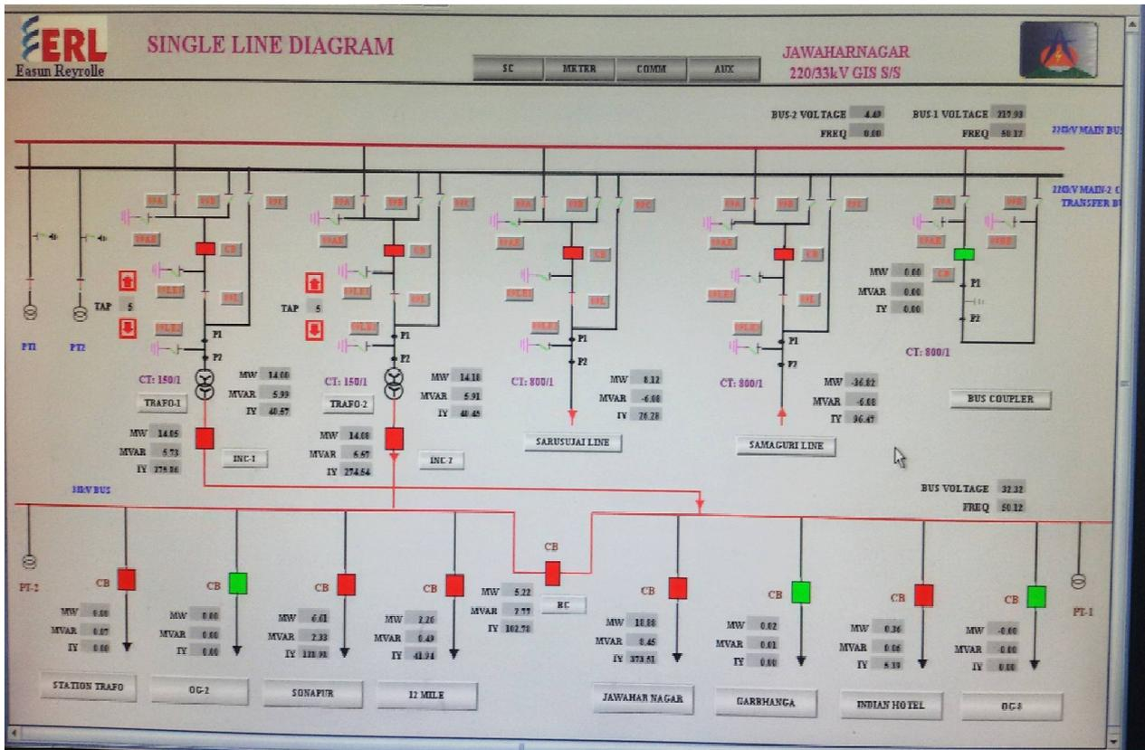
Fig.2: Single line diagram of GIS, Khanapara
