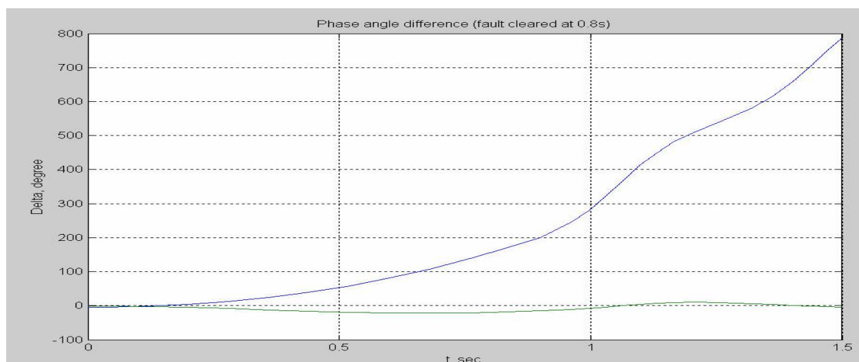
Fig. 3 Multimachine Stability for Fault cleared at 0.8 sec
