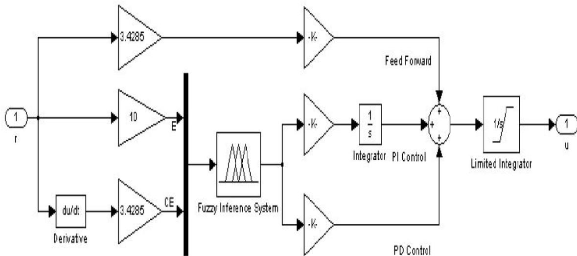
**Fig.2. Simulation of Fuzzy PID Controller**
