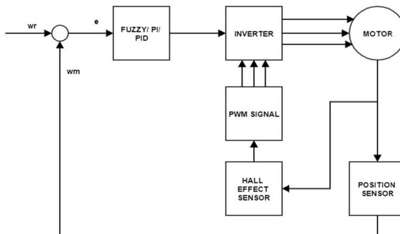
**Fig.3. Basic block diagram of proposed system**
