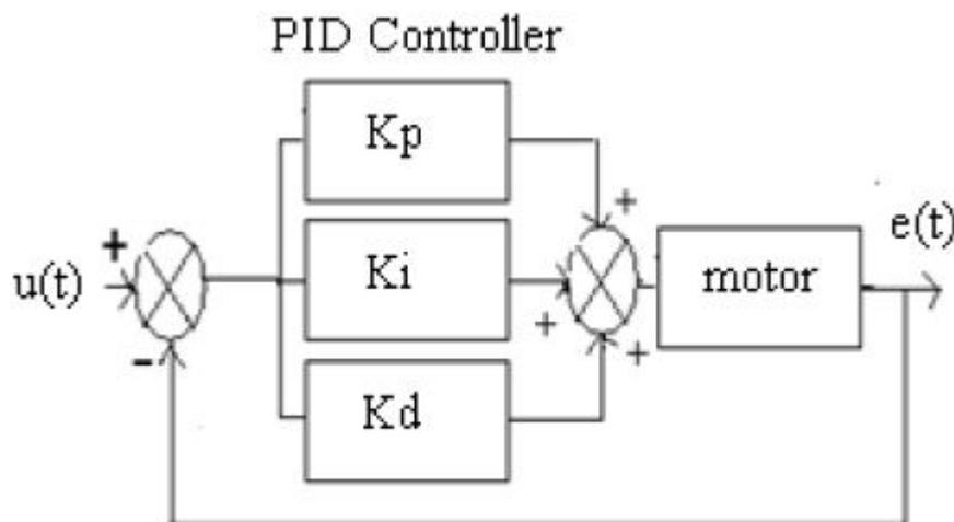
Fig 1. PID controller
