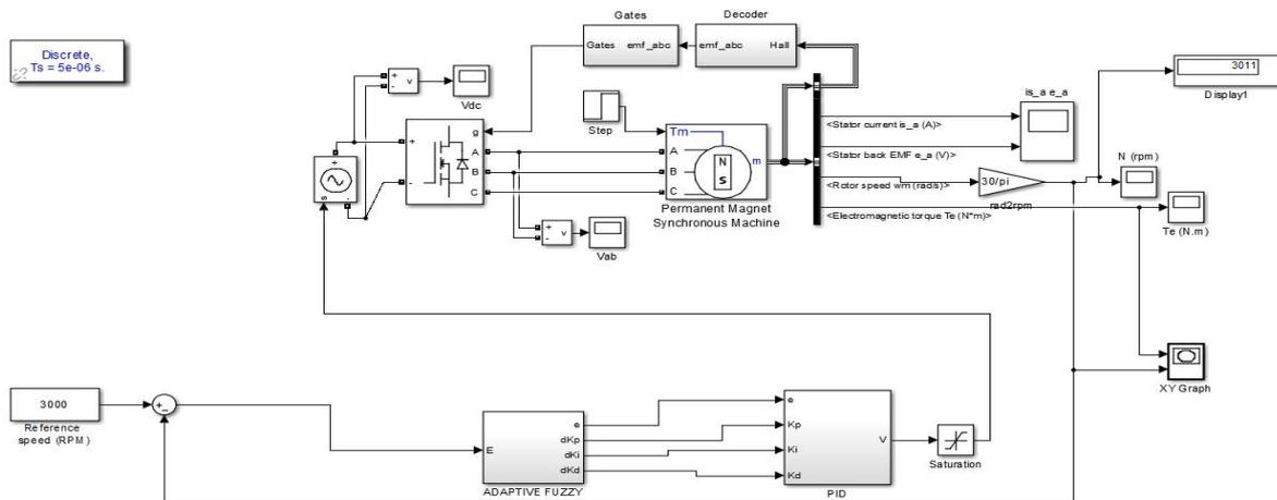
**Fig.4 Adaptive Fuzzy PID Controller**
