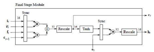
Figure 4: The module that computes the ct and ht from the results of the gates. is element-wise multiplication.
