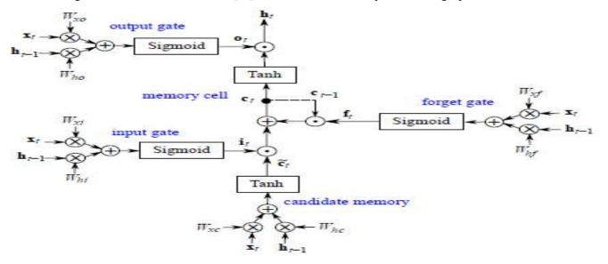
**Figure 2**: The vanilla LSTM architecture that was implemented in hardware represents matrix-vector multiplication and is element-wise multiplication.
