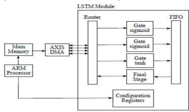
Figure 5: The LSTM module block diagram. It is mainly composed of three gates and one final stage module.
