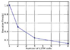
**Figure 8**: The execution time is projected to decrease with the increase of number of LSTM cells running in parallel. This can lead to significant performance improvement.
