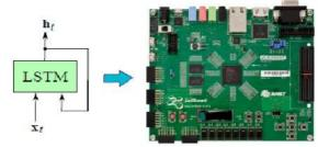
Figure 1: The LSTM hardware was implemented using a Zed board Zynq ZC7020.
