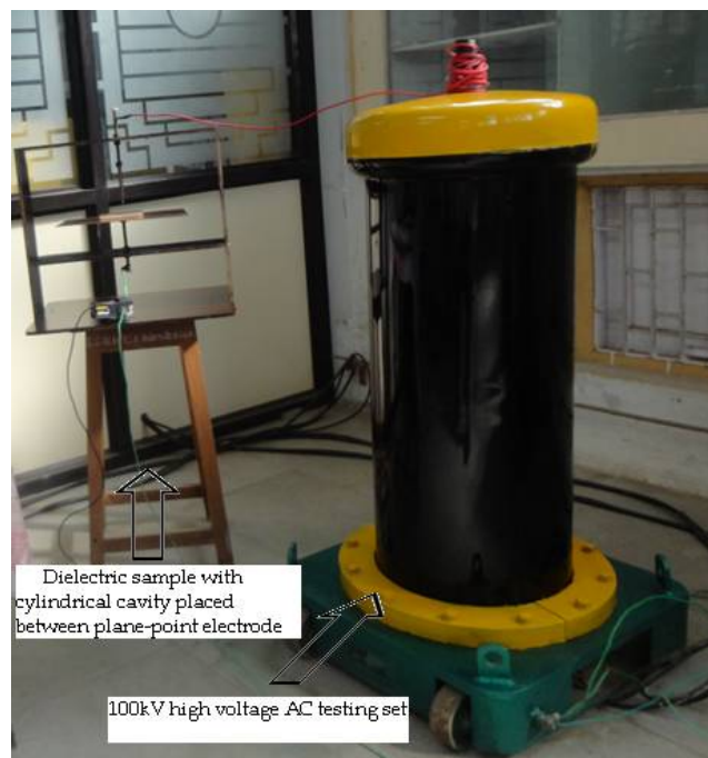
Fig. 3: Point-Plane Electrode Sample with 5mm gap
