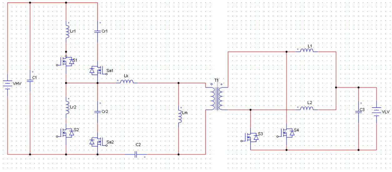
Fig. 1 Circuit diagram of soft switched isolated bidirectional converter
