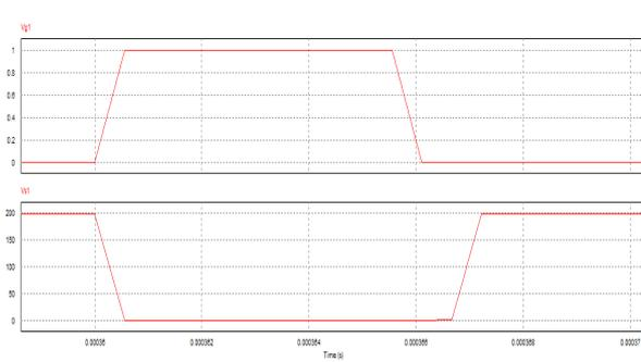
Fig. 7 ZVS turn off of the switch  $S_1$
