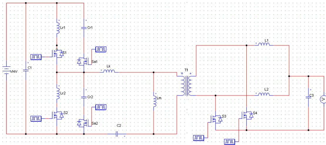
Fig. 3 Circuit diagram of soft switched isolated bidirectional converter in step down stage
