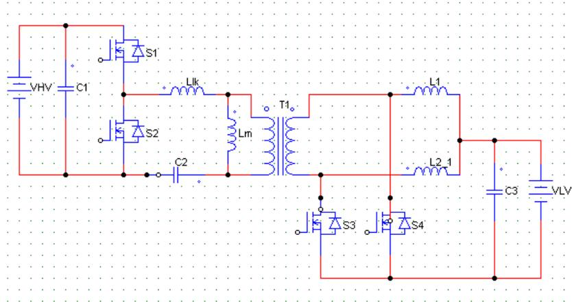
Fig. 2 Circuit diagram of isolated bidirectional converter
