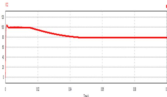
Fig. 6 Voltage across  $C_2$  during step down stage
