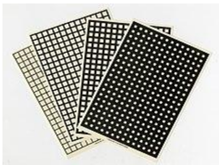
Ringelmann charts were developed for measuring smoke from chimneys and smokestacks at the end of the 19th century.
