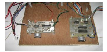
Fig.3. Ultrasonic Transmitter-Receiver Module
