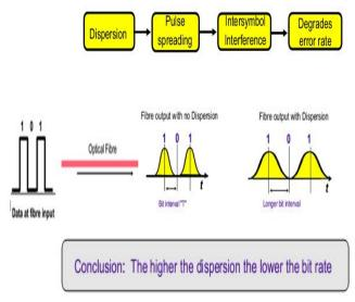
Fig.3: Dispersion in optical fiber [2]
