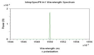
Fig.9: Input signal in frequency domain (N=1)
