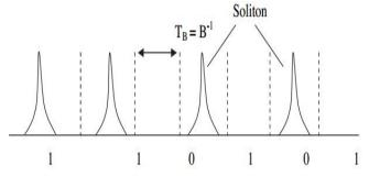
Fig.5: Soliton bit stream in an RZ format [3]
