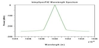
Fig. 18: Output signal in frequency domain (without soliton parameter) (N=3)
