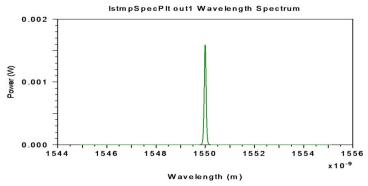
Fig. 15: Input signal in frequency domain (N=3)
