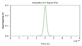
Fig.14: Input signal in time domain (N=3)
