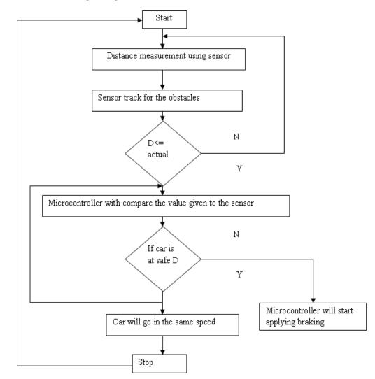
Fig. 5 Flow diagram of detecting obstacle
