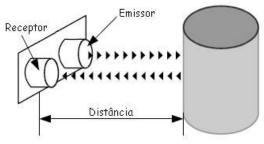
Fig. 3 Principle of ultrasonic sensor
