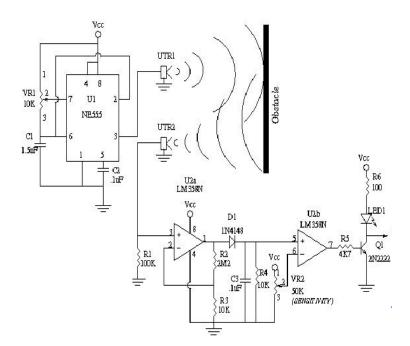
Fig. 4 Circuit diagram of ultrasonic sensor
