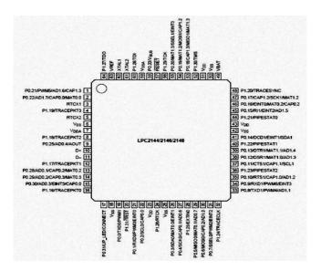
Fig. 2 Pin diagram of LPC 2148
