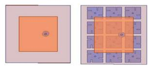
Figure [1] conventional antenna and antenna with FSS
