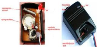
Fig 4.7: Piezo Electric Vibration Sensor
