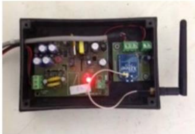
Fig.9. Transceiver unit to interface with base station
