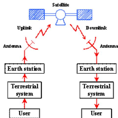
Figure 1. Block diagram of satellite communication
