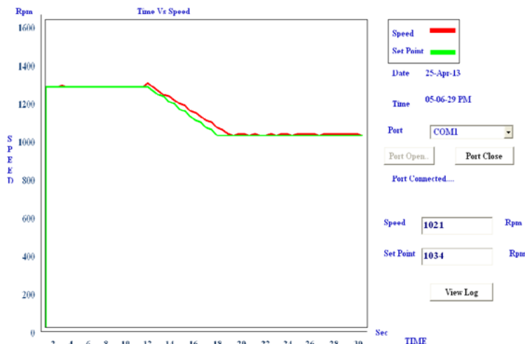
Figure 8 Transient State Performance Speed Varies 1300 to 1034 RPM
