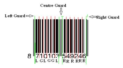
Fig .2 Decoding EAN-13
