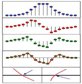
Fig .7 Steps in sub-pixel edge detection
