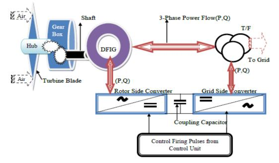
Fig. 1DFIG with power converter.
