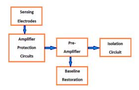
• Protection circuit: This circuit includes protection devices so that the high voltages that may appear across the input to the
