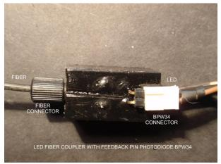
Fig.10 Photograph of LED-Fibre coupler with feedback PIN photodiode BPW34.
