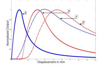
Fig. 3 Simulated responses with geometrical approach and measured output responses of optical fibre sensor obtained with plane and convex reflectors for air (RI=1). A- Simulated response with geometrical approach for convex reflector, B- Simulated response with geometrical approach for plane reflector, A'- Measured response for convex reflector, B'-Measured response for plane reflector.
