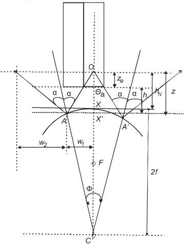
Fig. 2 Geometry of the light intensity modulation mechanism using a pair of optical fibres with a convex reflector.
