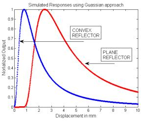
Fig. 4 Simulated output responses of optical fibre sensor obtained by Gaussian approach for plane reflector and convex reflector for refractive index = 1. The blind region of the sensor having convex reflector is zero, while plane reflector has a blind region.
