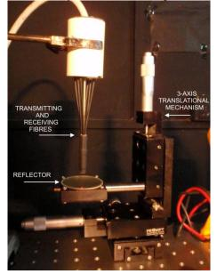
Fig. 7 Optical setup for the experiment with backlash free 3-axis translational mechanism.
