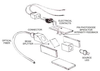
Fig.9 The mechanical assembly LED-Fibre coupler with feedback PIN photodiode BPW34.
