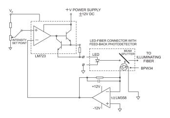
Fig. 8 LED stabilisation circuit with LED-Fibre connector with feed-back PIN photodiode BPW34.
