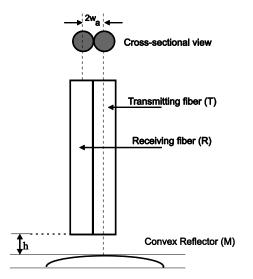
Fig. 1 The basic configuration of two fibre displacement sensor with convex reflector.Sensor.
