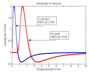
Fig. 5 The plot of sensor sensitivity versus displacement. The dead zone or blind region is absent in optical fibre sensor with convex reflector.
