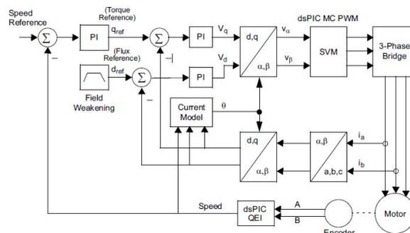
Fig. 1 Vector Control Block Diagram
