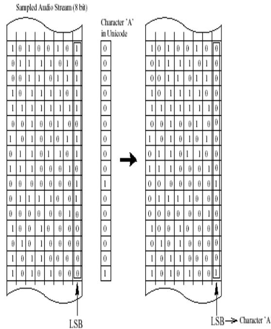
Fig 1: LSB encoding
