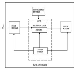
Microcontroller system Layout and connection
