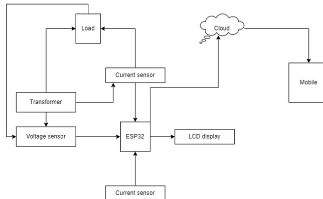
The LCD display can be used to display the power consumption data locally. The transformer is used to step down the voltage from the mains supply to a safe level for the ESP32 microcontroller.
